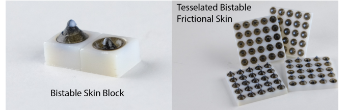
Fig. 4: Bistable skin blocks and bistable robotic skins are printed with a multi-material inkjet 3D printer. The black/dark parts are printed from high-frictional flexible Tango Black Plus. The white/light parts are printed from low-frictional rigid Vero White.
